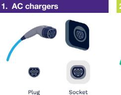
Australia uses Type 2 (for vehicles manufactured and sold after 2018). This is the plug used for all current vehicles imported into Australia. Type 2 is the standard plug compatible with AC chargers.
