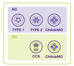
For EVs pre-2018 the Type 1 plug is most common. Current Mitsubishi PHEVs and Nissan Leafs, whilst compatible with Type 2 plugs with AC chargers, will need to use the CHAdeMO plug for faster DC chargers.
